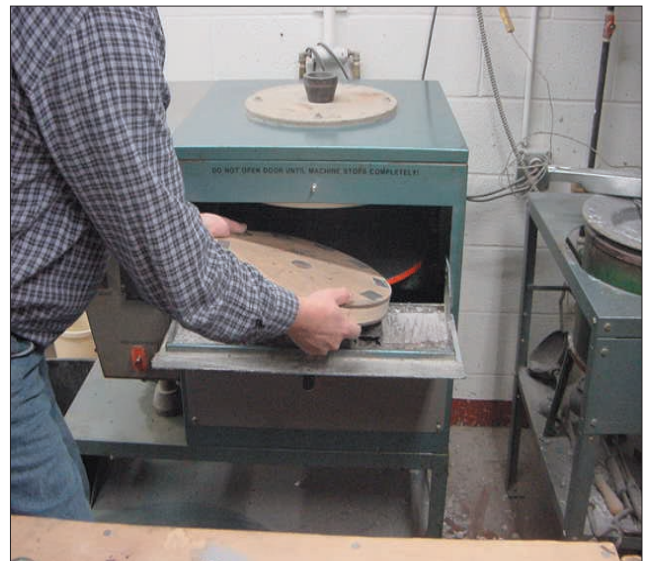
STEP 4 - Load the mould in spinning casting machine.
