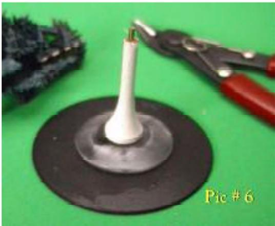
If you model was like mine, the remains of the broken plastic stem were still in the mount hole of the model. Use the 3/32 in. bit and drill a new mount hole into the remaining plastic. Apply super glue to brass and top of the golf tee and insert into the mount hole of the model. Support the model in position for a couple of minutes 'til the glue sets up.
